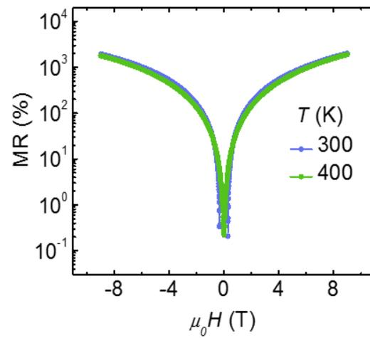
Graph of MR as a function of magnetic field strength  $H$  at 300 K and 400 K
