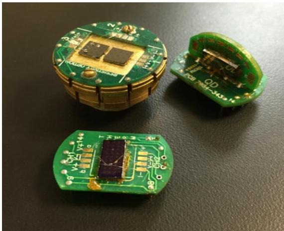
Prototypes of graphene-based magnetoresistance sensor
