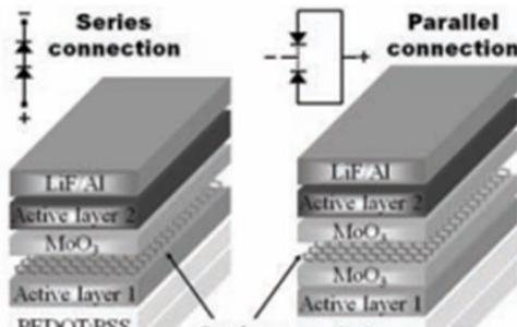
Schematic diagram of structures of photovoltaic devices: series and parallel arrangements
