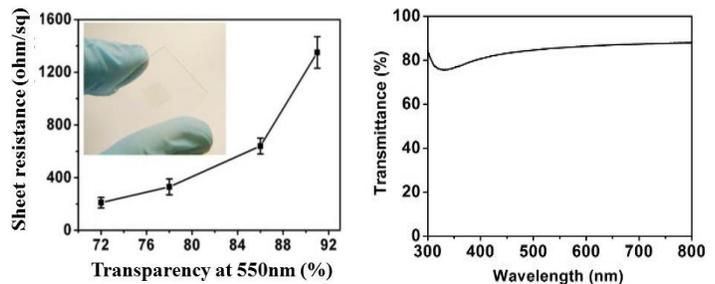
(a) High optical transparency at close to 90% with sheet resistance of 1350 ohm/□; (b) around 80% transmittance across 300 to 800 nm wavelengths
