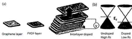
Fig 1: Working principle of graphene-based saturable absorber, showing the excitation process in (a) pristine graphene and (b) heavily p-type doped graphene; Fig 2: (a) Stack of graphene-ferroelectric PVDF layers; (b) band structures of undoped and doped graphene
